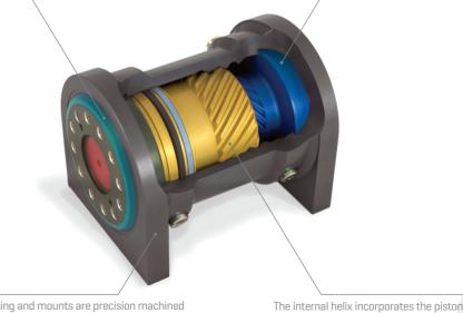
The housing and mounts are precision machined and treated witha surface hardening and corrosion resistant process
