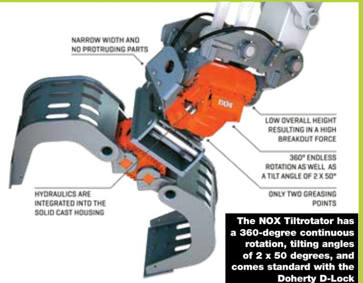
**The NOX Tiltrotator has a 360-degree continuous rotation, tilting angles of 2 x 50 degrees, and comes standard with the Doherty D-Lock**
