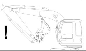
The installation of a quick coupler effectively lengthens the reach of your excavator's dipper arm. This may enable various attachments to come into contact with the boom set and operator's cabin. Operators must be aware of this and take appropriate care.
