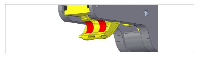
There are three wear areas that could be causing contact. It may be one area that is worn excessively or any combination of all three areas. All three areas should be checked and rectified if the below wear limits are exceeded.
