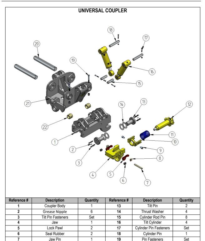
Always quote make and model of excavator and serial number of coupler when ordering parts, this is a reference guide only.
