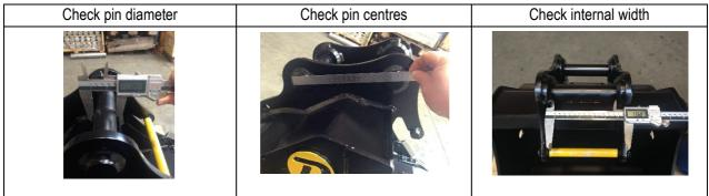
Note, Internal width should not exceed the width of the coupler more than 4mm per side. If coupler is used on under cutters, rock saws or any other attachment which has a significant side load the coupler MUST be a tight fit.
