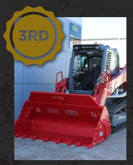
Based on proven results for the Australian made Norm Engineering 4in1 Loader Style Bucket, the floor is extended, side heights increased, and adding a higher load guard increased capacity.
