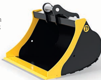
Powerdig mud buckets have a direct mount design with removable pins and short tip radius to provide maximum breakout force
