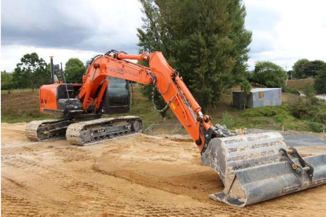
Photo: Bowe Brothers Excavating prepping a Waikato subdivision with the Doherty Tilt coupler and 3M wide bucket.
