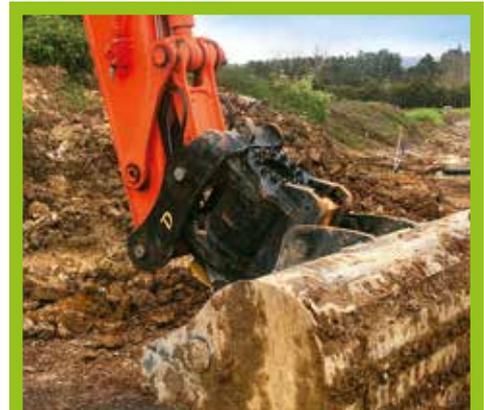
**The business end of the excavator housing a Snaplock+ Tilt provides an impressive 140 degrees of tilt along with a 1.8-wide Doherty cleaning bucket**
