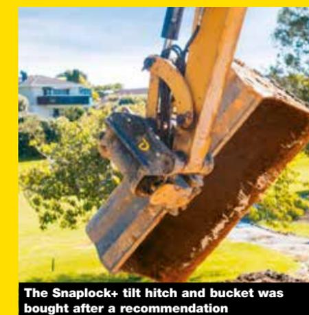
The Snaplock+ tilt hitch and bucket was bought after a recommendation
