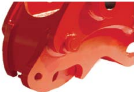
No safety pin hole
